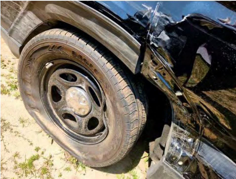
File Name / Description: DAMAGE_RT_RR_SUSP
