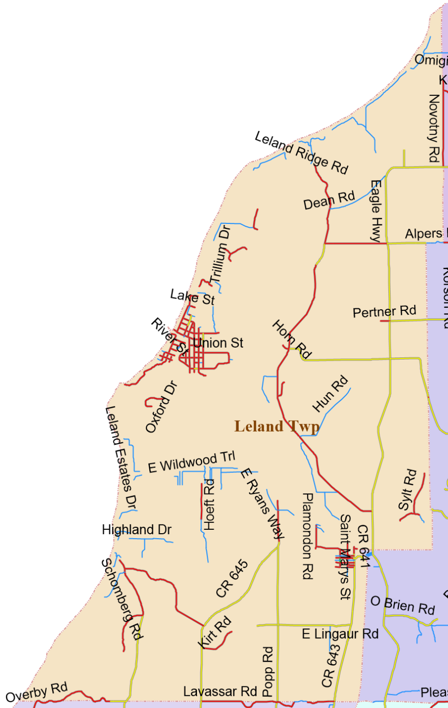
Figure 3: Leland Township Roads by PASER Rating Green = Good (8-10), Yellow = Fair (5-7), Red = Poor (1-4), Blue = Unrated
