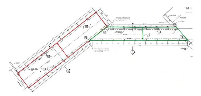
The first step for the removal will be to start removing the deck boards and sleepers in section 1 starting far left and working towards the right side. Gates and other miscellaneous items will be removed as well at this time. Items removed will be hand carried across the walkway and down the path to the roadway. These items will then be loaded on the forks of a telehandler and taken to the marina where they will be dumped into a waste dumpster.
